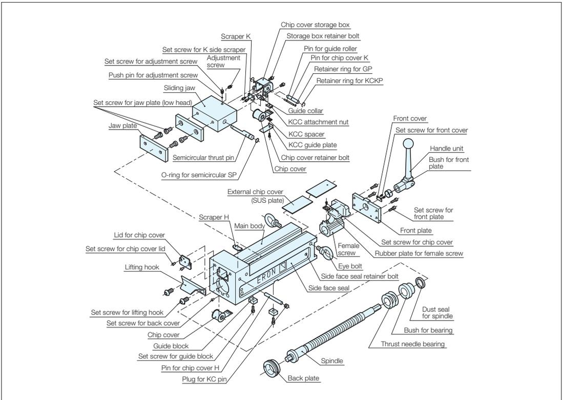
Jig Set-up Systems (Q-lock)
