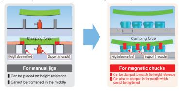
Jig Set-up Systems (Q-lock)
