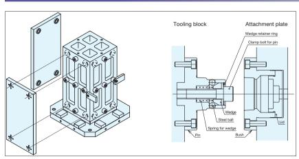
Jig Set-up Systems (Q-lock)
